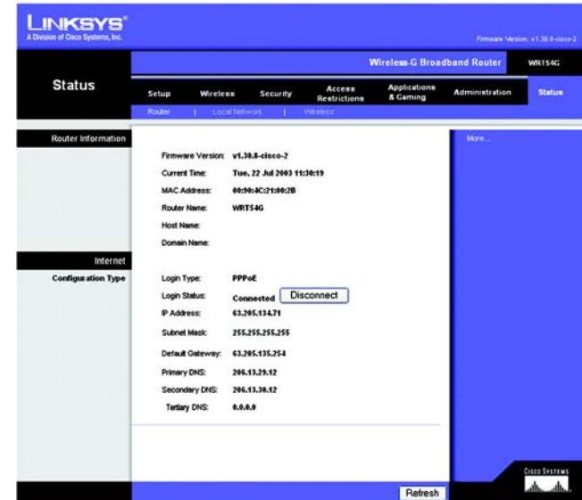
Figure 5-45: Status Tab - Router
